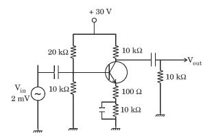
The output voltage,  $\mathbf{V}_{\text{out}}$  is nearly :
