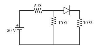
The minimum power rating of the diode should be:
